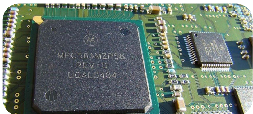
An MPC561 microprocessor, part of a family widely used in aerospace
